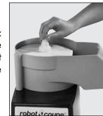
4) Then choose the disc to be set onto the ejecting plate.
