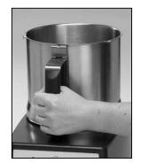
2) Turn the bowl to the right until the motor base connectors are securely positioned in their sockets. The magnetic rod should now be straight in front of you, in contact with the front of the motor base.
