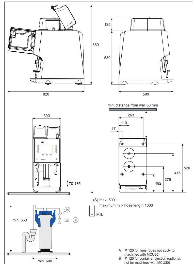
The Melitta® Cafina® XT4 is delivered ready for connection. However, before setting it up, the connections required on site must have been installed so that they are easily accessible within a radius of 1 m. This preliminary work must be carried out by authorized specialists in compliance with the applicable regulations. Melitta® Customer Services is not authorized to carry out this work and does not assume any responsibility for the installation.
