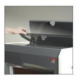
Rear safety cover Closing it initiates the slicing process and the machine stays mechanically and electrically locked during cutting.
